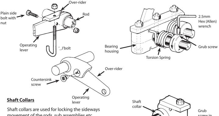
movement of the rods, sub assemblies etc. Tighten the grub screw with the 2.5mm Hex wrench (Allen Key) to lock the collar in position ensuring that the rods etc, rotate freely.
