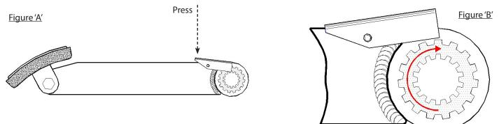
To **raise** the height of the pedal rotate the splined collar 1 or 2 teeth in a clockwise direction as figure 'B', re-fit the pedal to check the travel & operation of the dual control pedals. Continue adjusting the pedal height with this method until the desired height is achieved. In order to lower the pedal height simply rotate the internal splined collar in a anti-clockwise direction.
