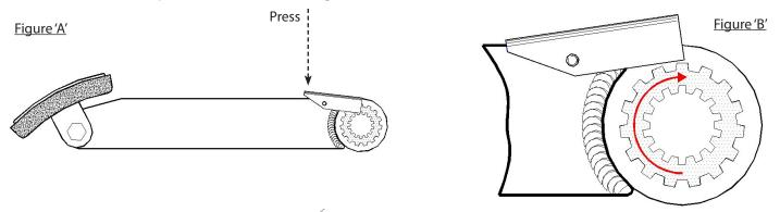
To **raise** the height of the pedal rotate the splined collar 1 or 2 teeth in a clockwise direction as figure 'B', re-fit the pedal to check the travel & operation of the dual control pedals. Continue adjusting the pedal height with this method until the desired height is achieved. In order to lower the pedal height simply rotate the internal splined collar in a anti-clockwise direction.
