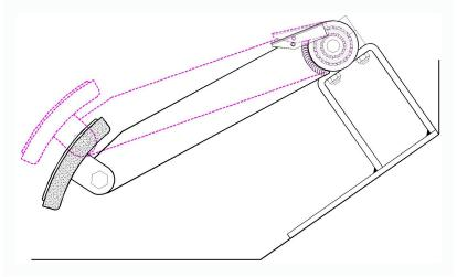
With the height adjustment complete re-secure the pedals to the rods.
