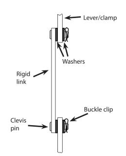
On some models that use rigid links, the clevis pin & buckle clips are replaced with M8 bolts with Nyloc nuts. The Nyloc nuts can be adjusted where the links connect to the levers & clamps to ensure that they pivot freely.
